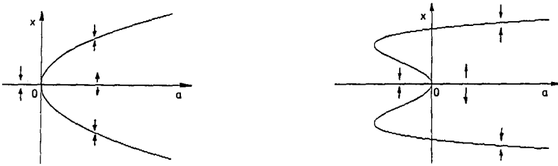
Fig.7. Supercritical and subcritical bifurcation of the stationary solution of Eq.(3.1) in the deterministic case.
